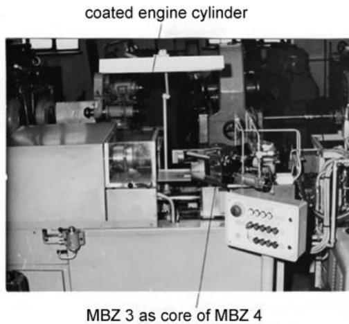
Figure 5 The brass-coating device applied in an automatic machine
