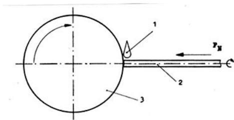
Figure 1 Scheme of copper deposition (1 - surface active liquid; 2 - brass rod; 3 - shaft to be coated)
