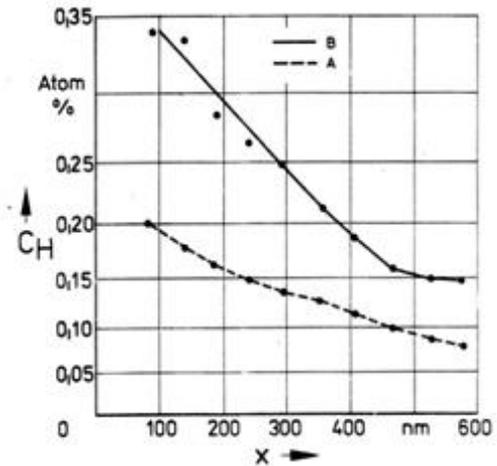
Figure 7 Reduction of  $H_2$  concentration at the frictional surface in depth
