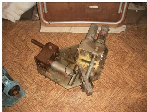
Figure 4 View of the brass-coating device MBZ 3A
