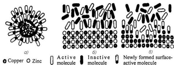
Figure 2 Formation of micelles and interaction of surface-active substances with bronze (as per [10])
