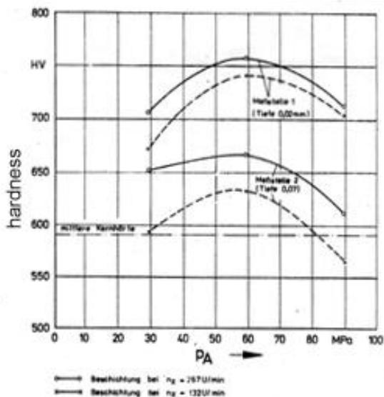
Figure 6 Hardness in different depth after frictional coating deposition on steel: meas. point 1 – depth 0,02 mm; meas. point 2 – depth 0,02 mm; continuous line: coating deposition at  $n_z = 267$  rev/min, dash line: coating deposition at  $n_z = 132$  rev/min
