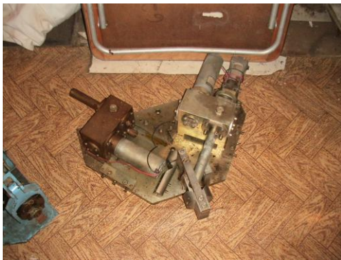
Figure 2 View of the brass-coating device MBZ 3A [7]
